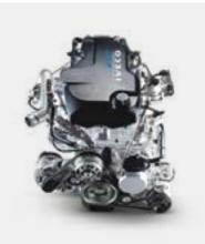
2.3-litre F1A diesel engine with SCR
