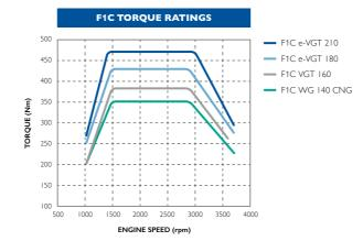
e-VGT: Electronic Variable Geometry Turbocharger; VGT: Variable Geometry Turbocharger; WG: WasteGate; CNG: Compressed Natural Gas
